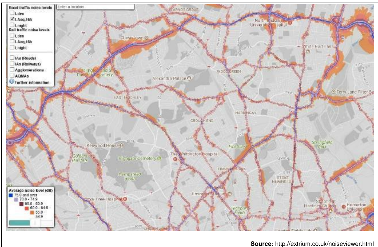
Figure 3.4: LAeq 16-hour road traffic noise levels in London Borough of Haringey 2012
